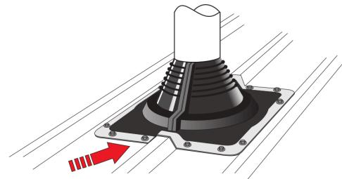
REALIGN FLASHING ONTO ROOF AND FIX WITH APPROPRIATE FASTENERS. START HERE.
