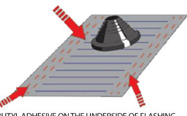
FULL BUTYL ADHESIVE ON THE UNDERSIDE OF FLASHING
