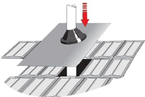
FORM AN ANTI-CAPILLARY FOLD AT TOP OF BASE SHEET
