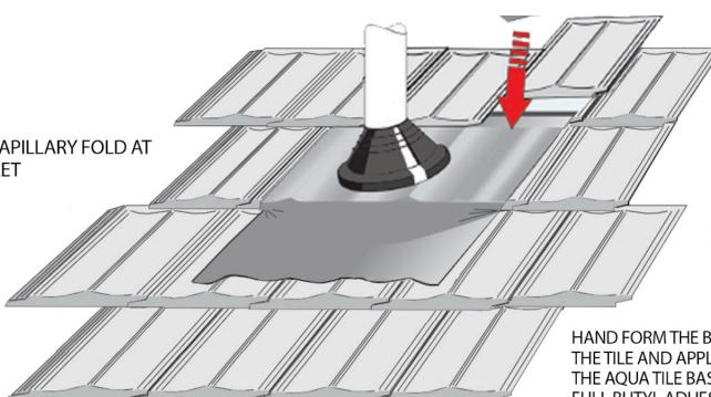
REMOVE THE REMAINING PROTECTIVE BACKING FROM THE UNDERSIDE OF THE AQUA TILE THAT IS COVERING THE BUTYL ADHESIVE
