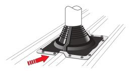
REALIGN FLASHING ONTO ROOF AND FIX WITH APPROPRIATE FASTENERS. START HERE.
