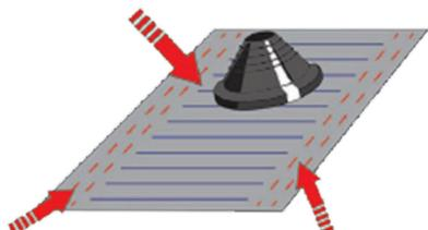
FULL BUTYL ADHESIVE ON THE UNDERSIDE OF FLASHING
