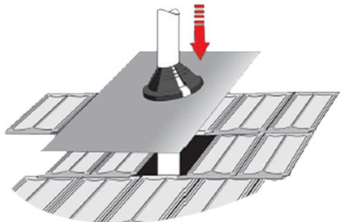
FORM AN ANTI-CAPILLARY FOLD AT TOP OF BASE SHEET
