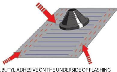
FULL BUTYL ADHESIVE ON THE UNDERSIDE OF FLASHING
