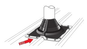
REALIGN FLASHING ONTO ROOF AND FIX WITH APPROPRIATE FASTENERS. START HERE.
